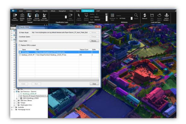
• Import and Convert Mesh Layers - TerraExplorer 7.1 extends mesh layer support to include the import and conversion of BIM and DAE formats to a stream-optimized 3DML.
